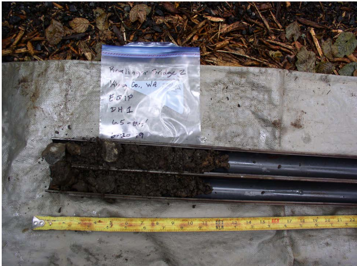
Figure 5. View of sample recovered from a depth of 6.5 to 8.0 feet.
