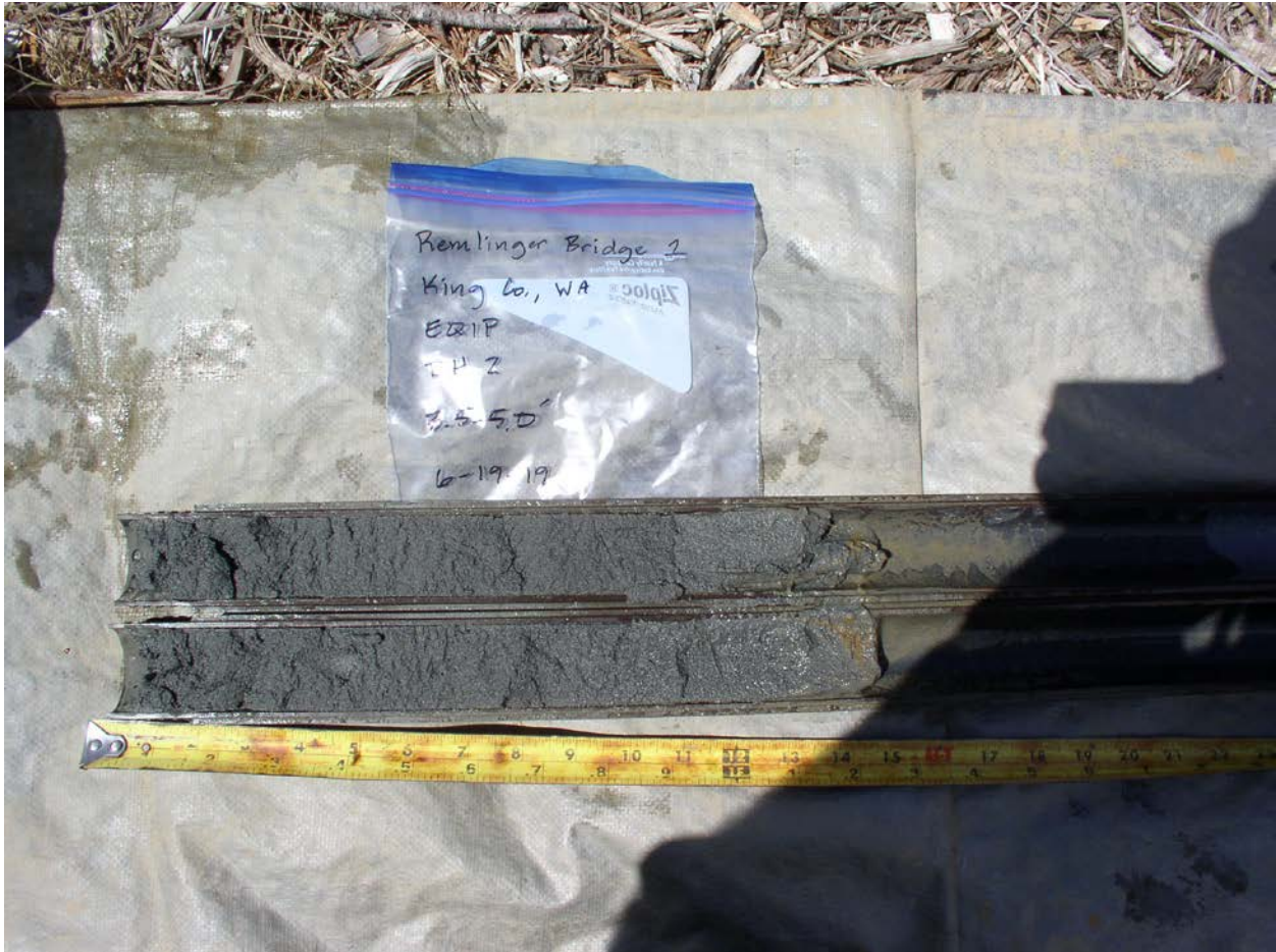
Figure 11. View of sample recovered from a depth of 3.5 to 5.0 feet.
