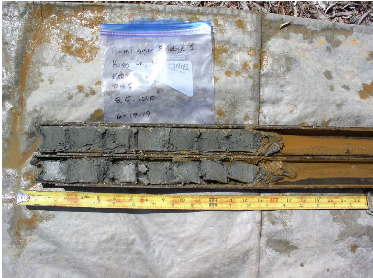
Figure 7. View of sample recovered from a depth of 8.5 to 10.0 feet.
