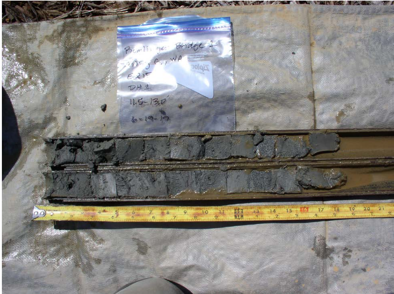
Figure 8. View of sample recovered from a depth of 11.5 to 13.0 feet.
