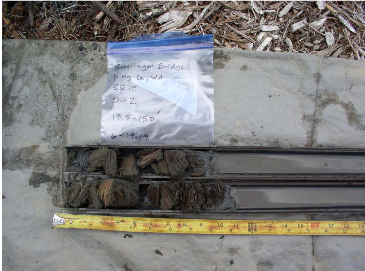
Figure 15. View of sample recovered from a depth of 13.5 to 15.0 feet.
