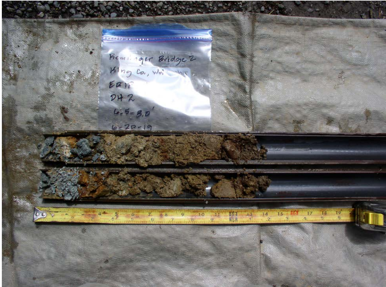
Figure 9. View of sample recovered from a depth of 6.5 to 8.0 feet
