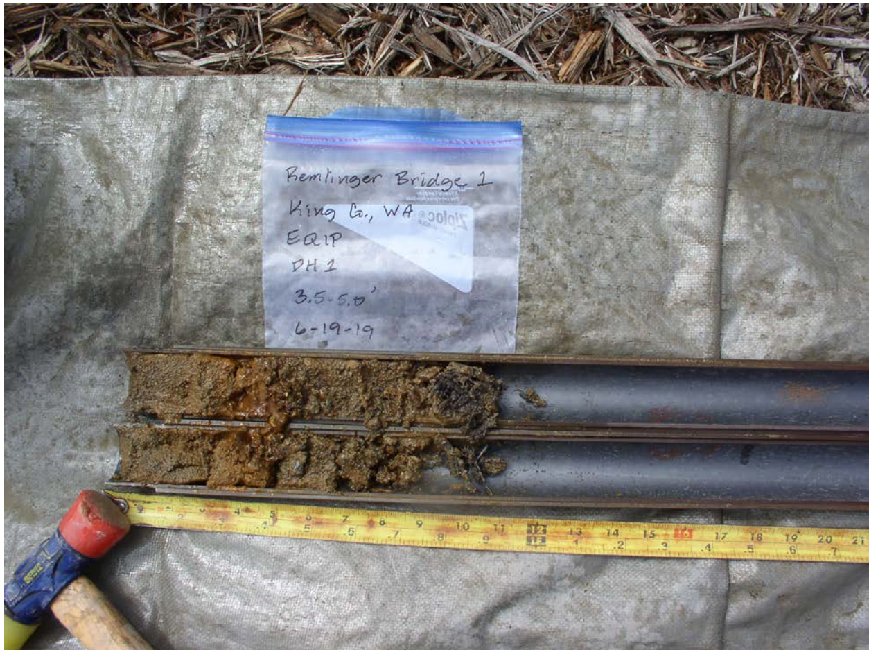
Figure 5. View of sample recovered from a depth of 3.5 to 5.0 feet.
