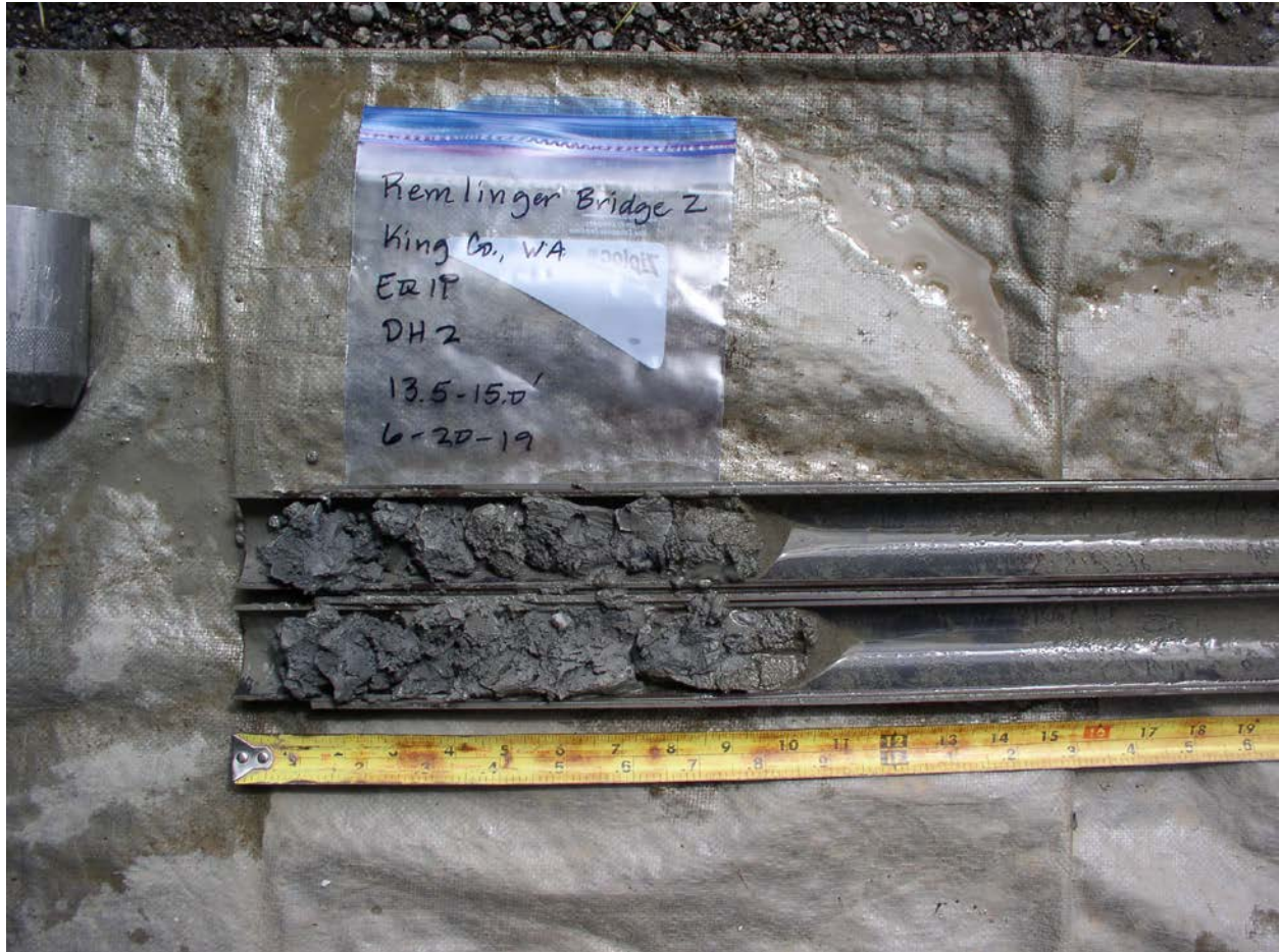
Figure 12. View of sample recovered from a depth of 13.5 to 15.0 feet.
