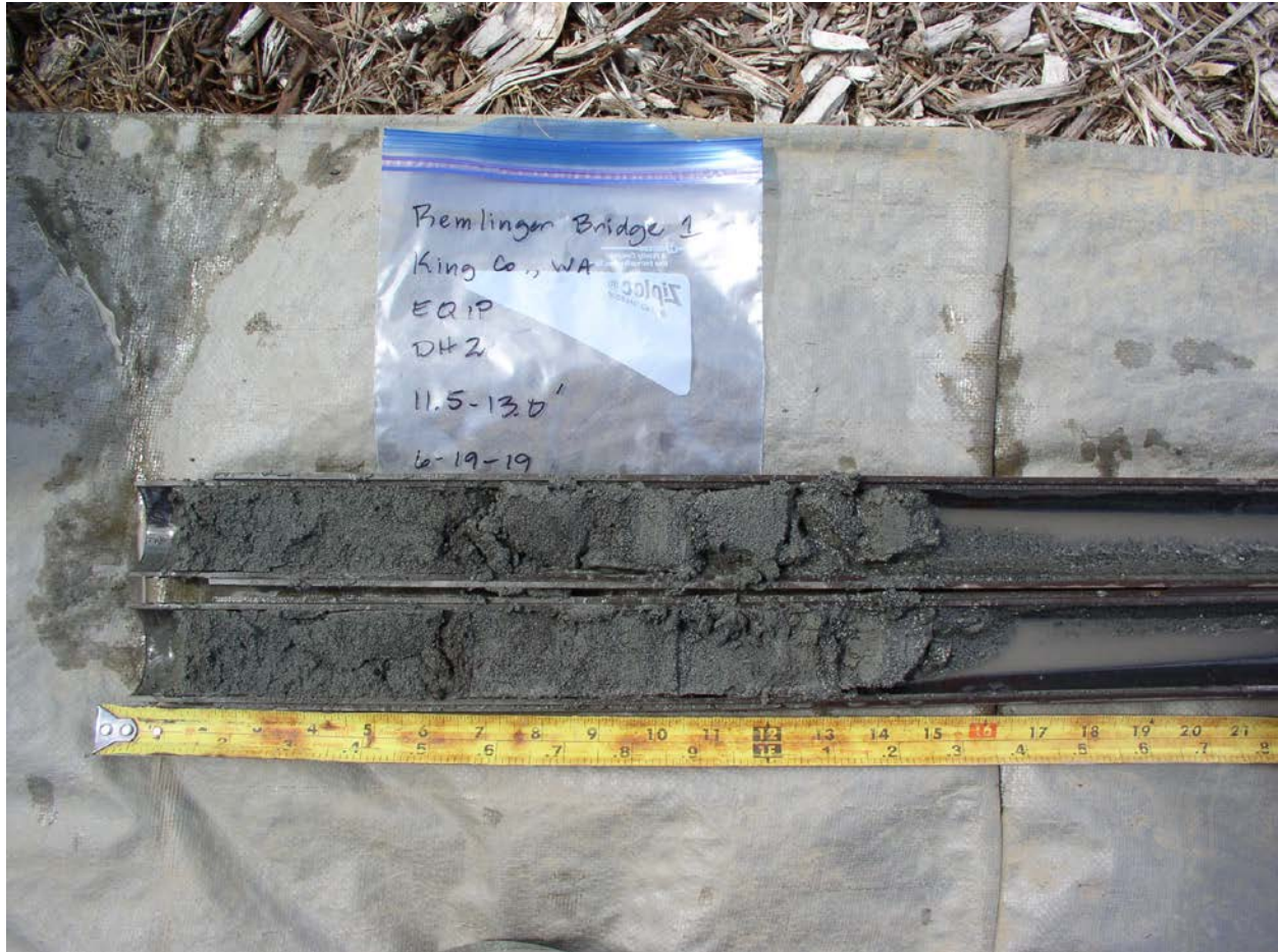
Figure 14. View of sample recovered from a depth of 11.5 to 13.0 feet.
