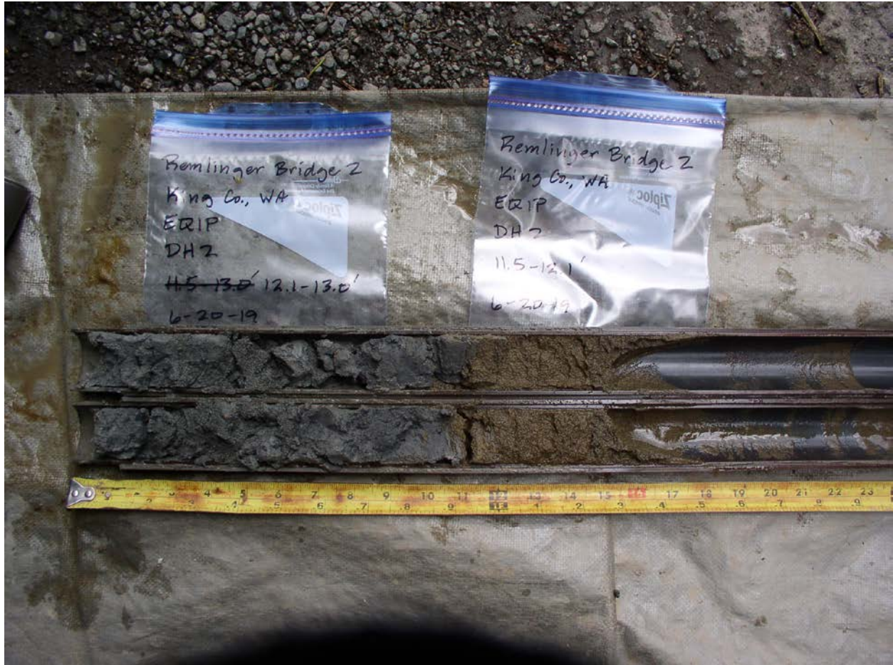
Figure 11. View of sample recovered from a depth of 11.5 to 13.0 feet.
