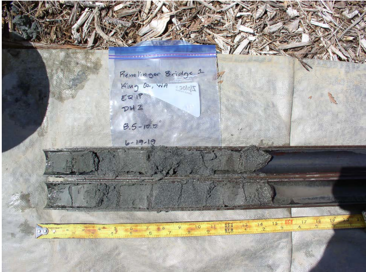
Figure 13. View of sample recovered from a depth of 8.5 to 10.0 feet.
