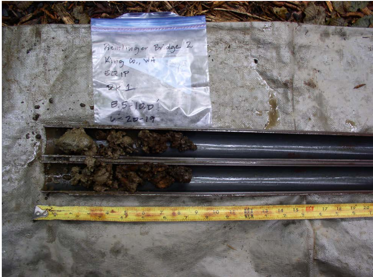
Figure 6. View of sample recovered from a depth of 8.5 to 10.0 feet.
