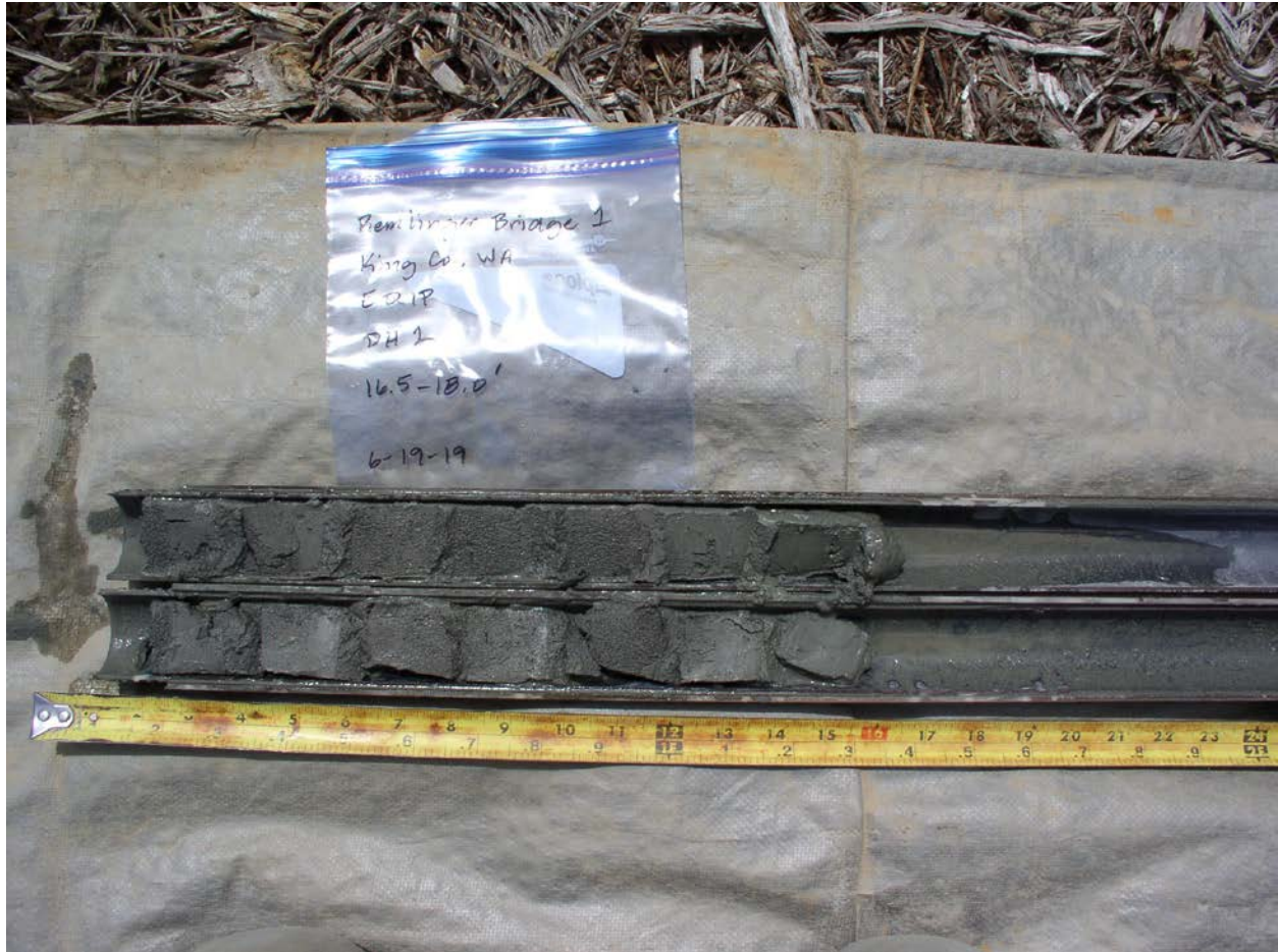
Figure 10. View of sample recovered from a depth of 16.5 to 18.0 feet.
