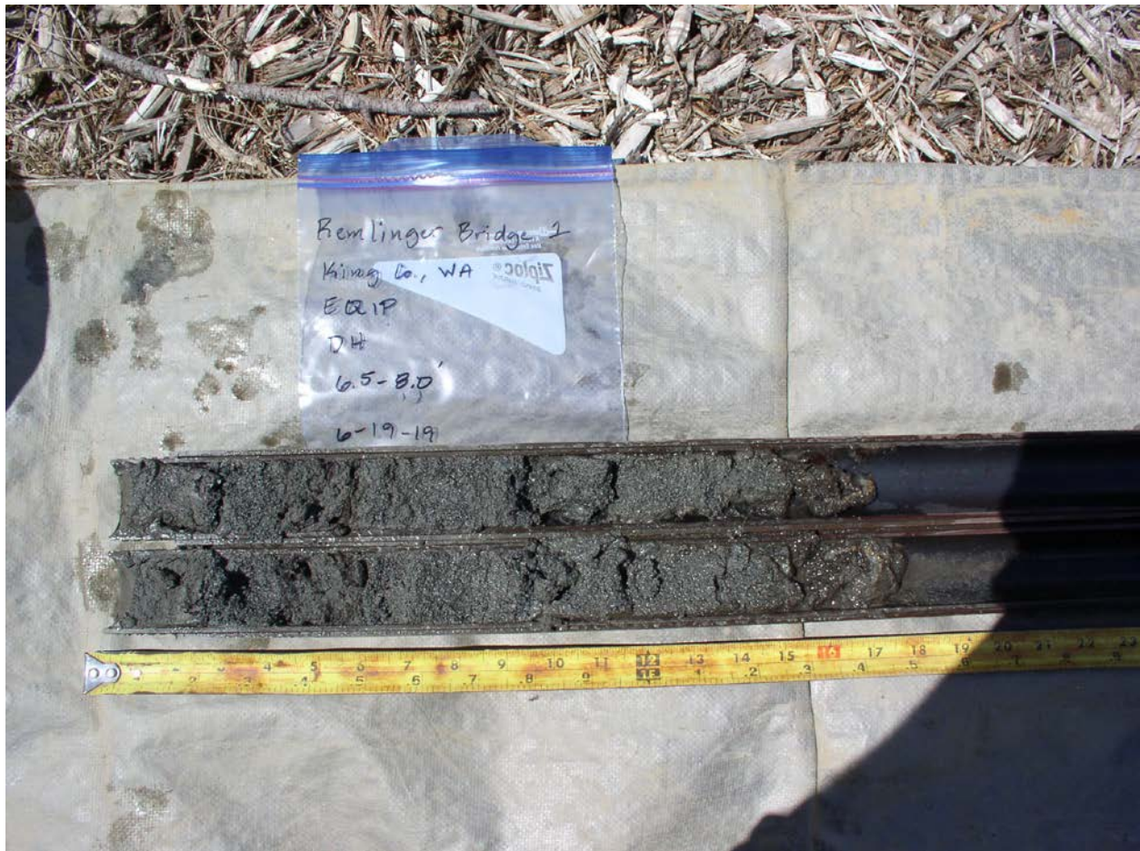
Figure 12. View of sample recovered from a depth of 6.5 to 8.0 feet
