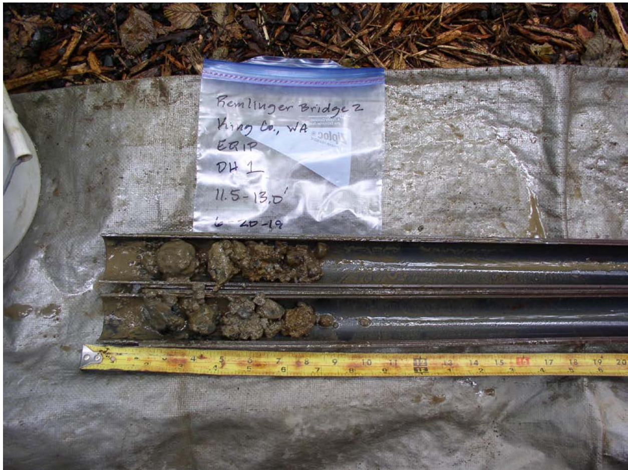
Figure 7. View of sample recovered from a depth of 11.5 to 13.0 feet.
