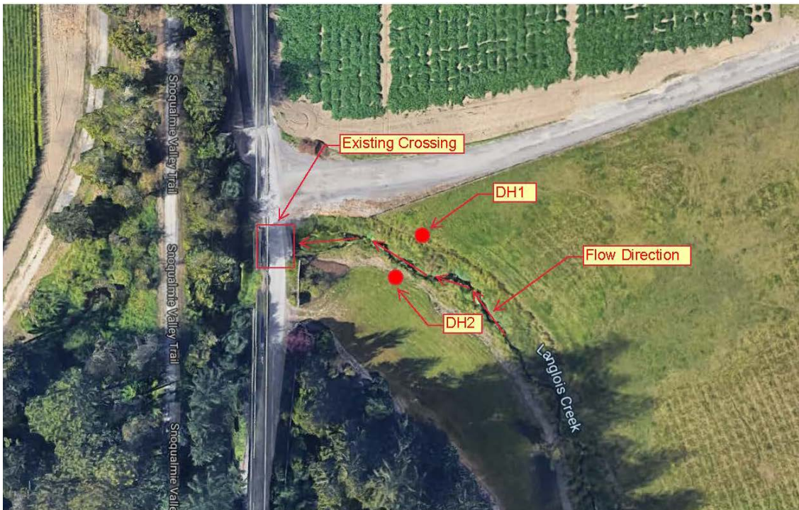
Figure 2. Aerial image of Remlinger Farms site 1 with the approximate location of the exploratory drill holes. North is towards top of page.
