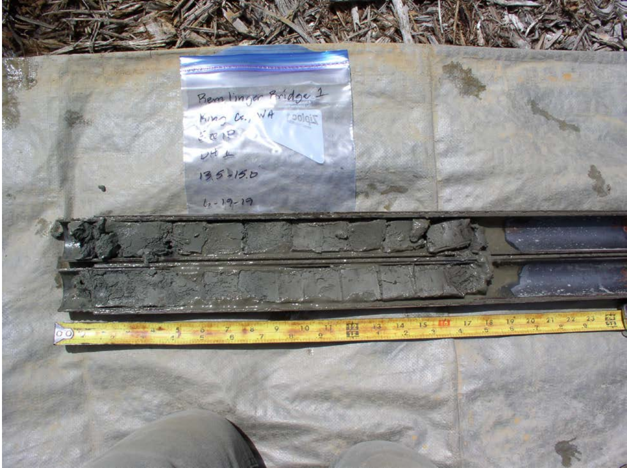
Figure 9. View of sample recovered from a depth of 13.5 to 15.0 feet.
